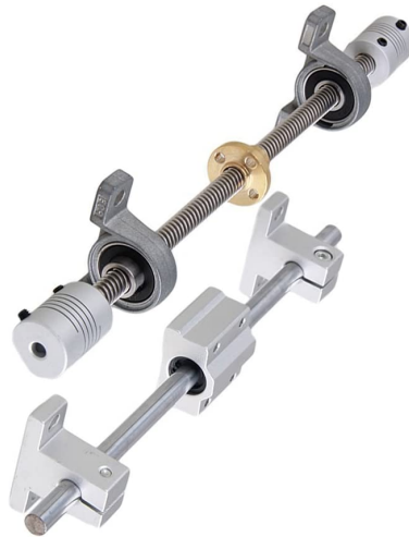
Figure 3.7: Acme screw set utilized to build the custom linear actuator for microscope/camera setup. Parts in the set include an 8mm acme screw, dual support rods, pillow bearings, support blocks, and brass nut. The support rods and acme screw were cut to size and fitted into 3D printed mounts.
