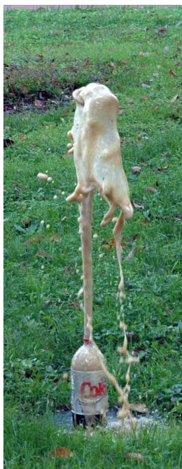
Figure 1. The fountain effect when 16 Mentos are placed in a 2-liter bottle containing Diet Coke.
