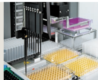
Simultaneous liquid handling and labware movement
