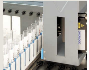
Identification of sample tubes prior to use
