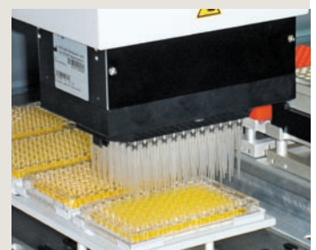
96-channel pipetting head for sample preparation
