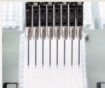
Pipetting into 1536-well plate
