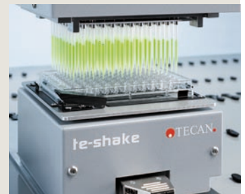
Sample transfer to a microplate while shaking
