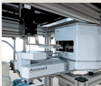
Robotic manipulator with extended Z-axis for access beneath worktable
