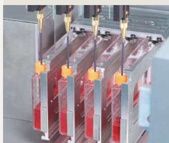
Tecan's Cellerity™ fully automated cell culture system pierces Corning® RoboFlask® septa
