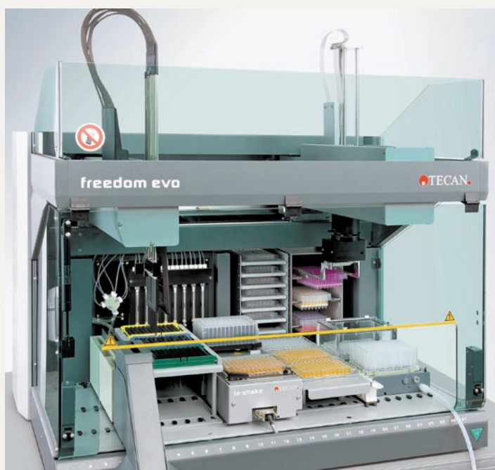
Nucleic acid sample preparation on a Freedom EVO 75
