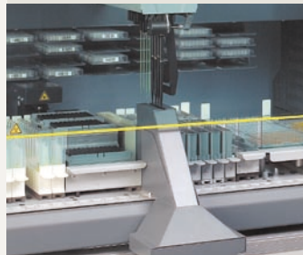
Low disposable tip ejection contains aerosol transmission
