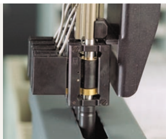
Low disposable tip ejection for aerosol-free disposal
