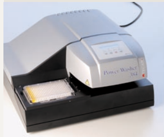
Power Washer for high-speed washing of 384-well and 96-well plates
