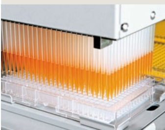
MultiChannel 384 Arm for high throughput plate-based applications
