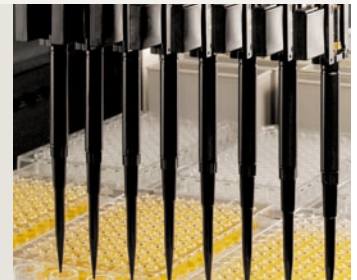
Tip spacing adjusts automatically between labware formats
