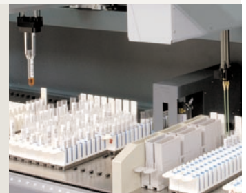
Automated tube identification and sorting
