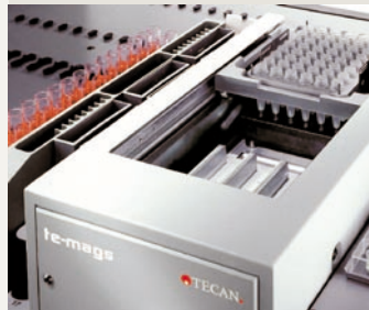
Te-MagS performs magnetic bead separation
