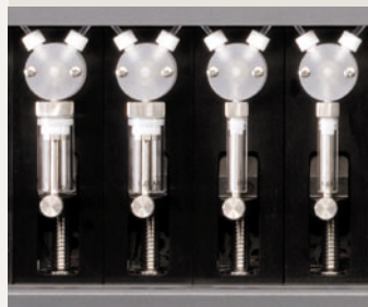
Syringe pump selection optimizes liquid volume range.
