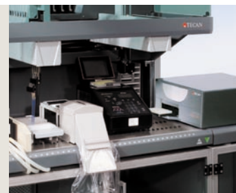
PCR application with integrated thermocycler and Tecan reader
