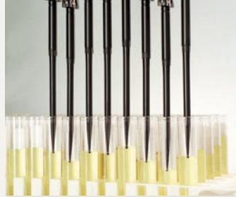
Liquid level detection in individual sample tubes
