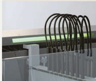
Status lamp clearly displays instrument status
