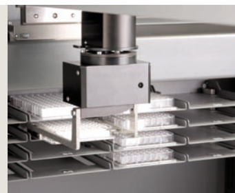
Robotic manipulator for microplate movements
