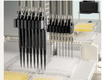
Combination of fixed and disposable tips on two liquid handling arms
