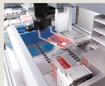
Automated expansion can be performed in plates, tubes or flasks
