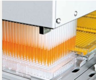
384-channel pipetting head
