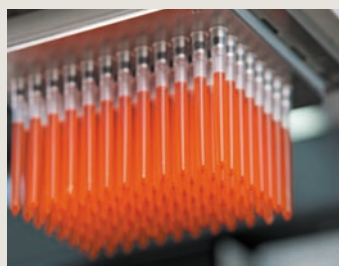
With the Extended Volume Adapter (EVA) the 384-channel head can pipette up to 500 µl in the 96 well format
