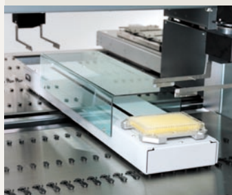
Plate transfer between two Freedom EVO platforms by Te-Link
