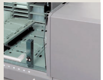
Personnel are protected by interlocked shields
