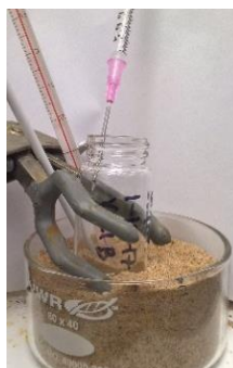
Figure 2. Extraction liquid reduction setup using a sand bath and 2 psi nitrogen stream.
