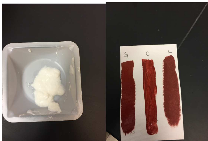
Figure 1. A (left). Picture of casein binder before pigment is added. B (right). Picture of strips of paint made with each binder.
