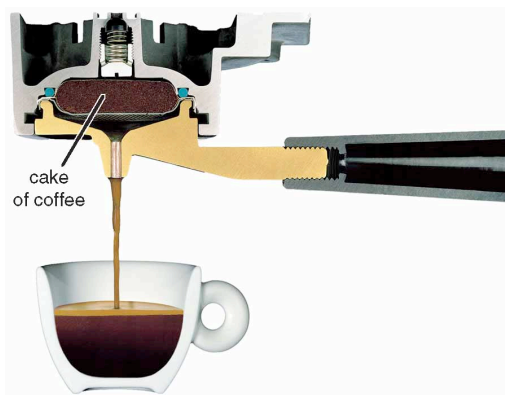
Figure 9. Cross-sectional detail of a typical espresso percolation device.
