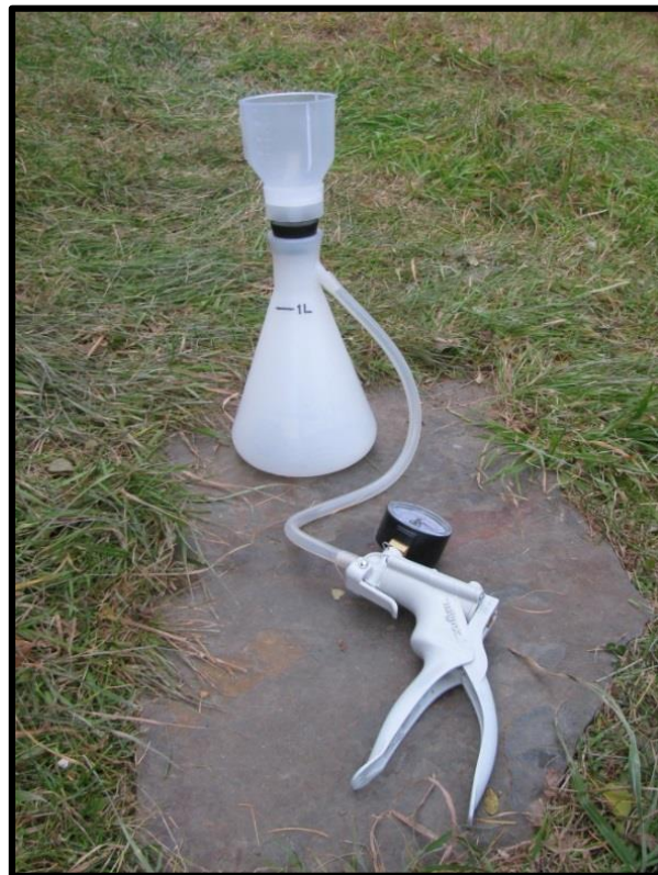
Figure 7. Filter assembly. Note pressure release lever on underside of vacuum pump near the nozzle.
