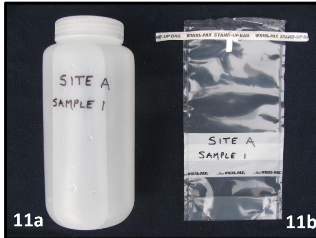
Figure 3. Polypropylene grab bottles (11a) and Whirl-Pak® bag (11b).
