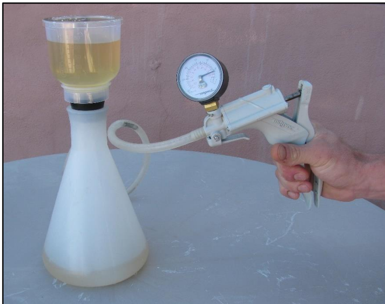
Figure 10. Engage hand pump to begin filtration.
