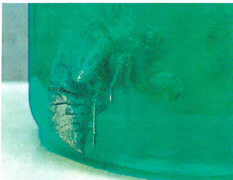
Figure 2. Pretreated cicada exoskeleton being plated in the electroless nickel plating bath at 85 °C. Note the bubbles of H 2 (g) emanating from its surface.
