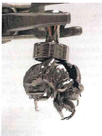
Figure 3. Nickel-plated cicada exoskeleton being held by a neodymium magnet.
