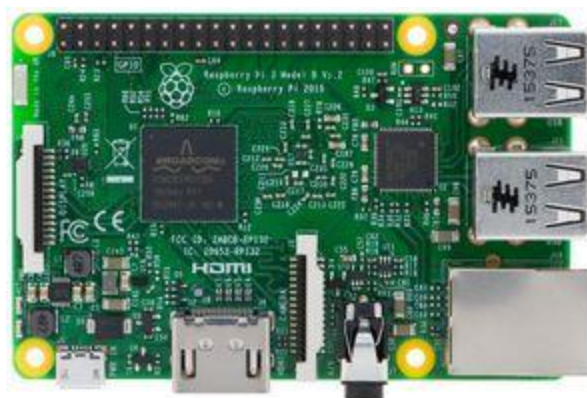
Figure 3. A Raspberry Pi 3 Computer
